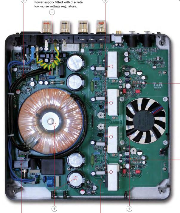
Sophisticated mains filtering to block RF interference and DC voltage.
