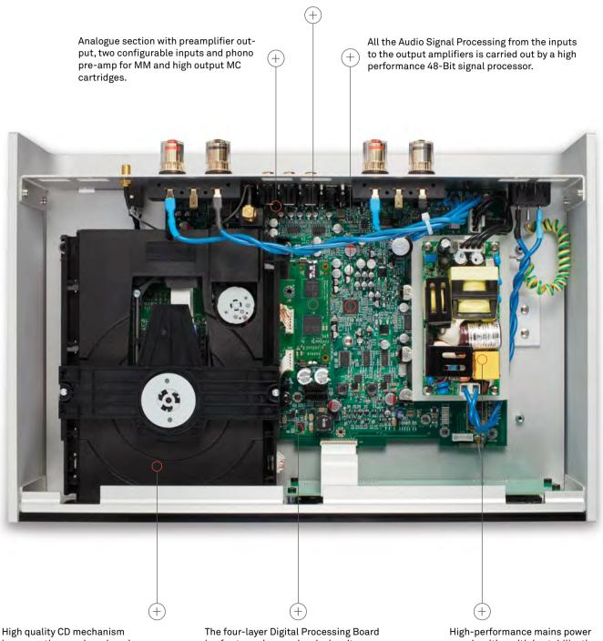
High quality CD mechanism incorporating modern decoder technology, offering very fast access times and excellent error correction.
